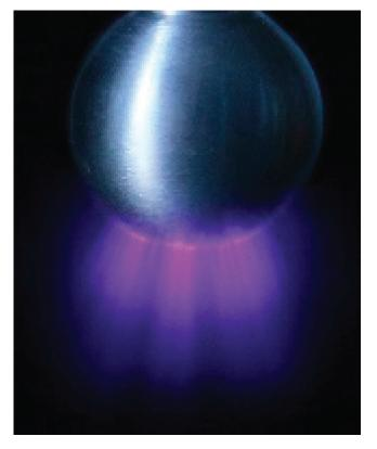
Figure 2. Direct-current corona discharge of negative polarity on a spherical surface, showing a stage with an amalgam of moving streamers blurring into a broad glow in blue to purple colours (from Riba et al., 2018, p. 10, fig. 4b).
